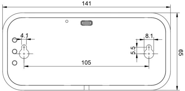
NIX4F drawing, viewing the back. All dimensions in mm, 1:1 scale – verify scale after printing.
